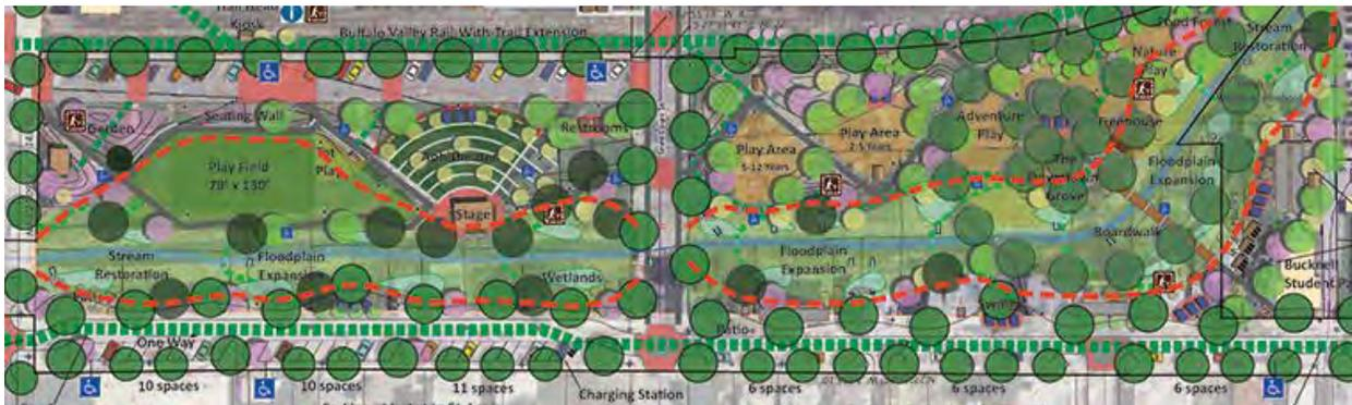
*The Bull Run Greenway will seek to restore the stream and reconnect the floodplain, improving the stream as a park amenity while increasing flood holding capacity. The dashed red line in the plan above delineates the extents of the expanded floodplain. Areas such as the play field lawn and nature play area will be designed to flood while providing better access to the stream.*
