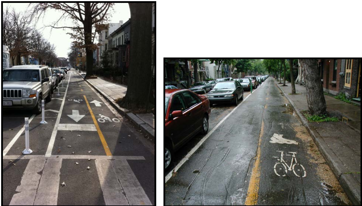
Figure 7.10 – Typical Cycle Tracks
