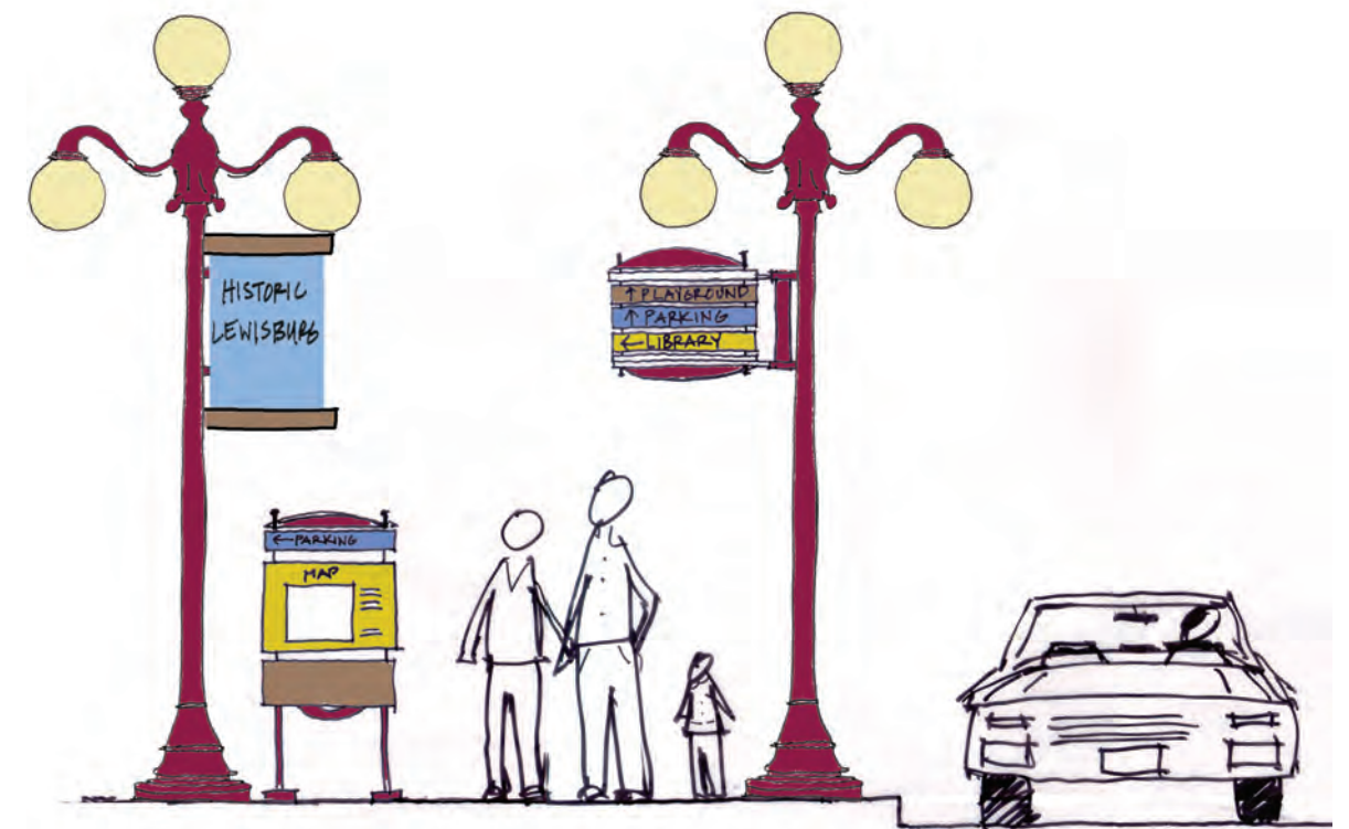
Figure 4.12: Driver and Pedestrian-oriented Wayfinding Signage for the northern half of the corridor.
