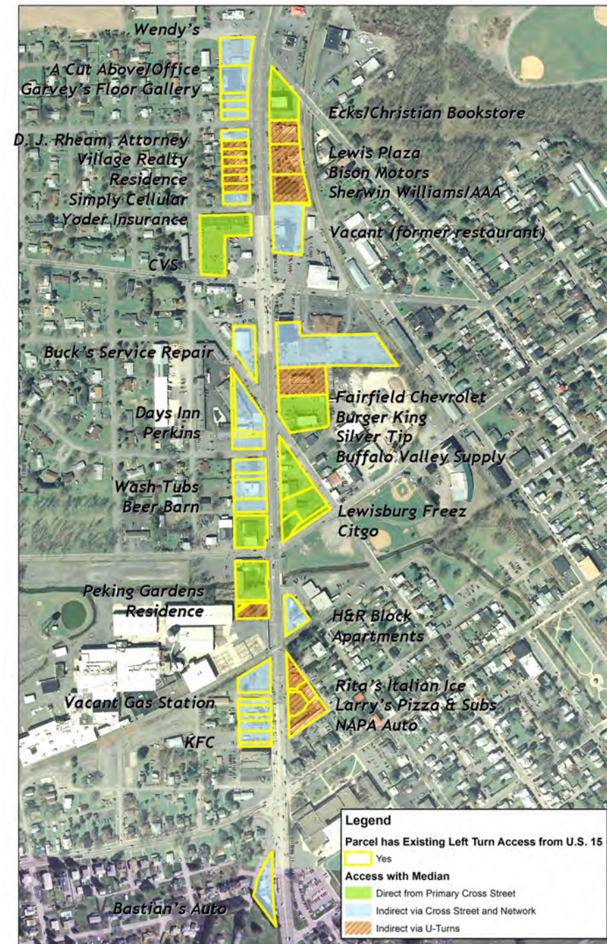
Figure 4.19: Modified Access Conditions along US 15 with Implementation of Green Median Concept: Parcels labeled according to type of access to / from US 15
